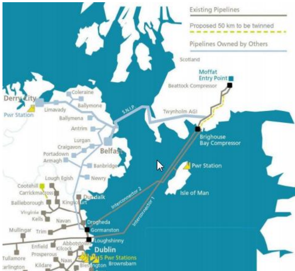
Figure 7. PCI 5.2 Twinning of Interconnector for 50km in Scotland which brings increased security of supply to Ireland with 2 completely independent interconnectors, representing 2 separate pieces of gas infrastructure
