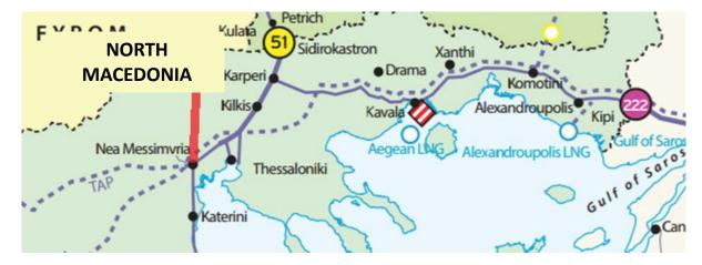
**Description**: The project consists of a 56 km, 28" or 30" pipeline, from Nea Messimvria to the Greece/North Macedonia border.
